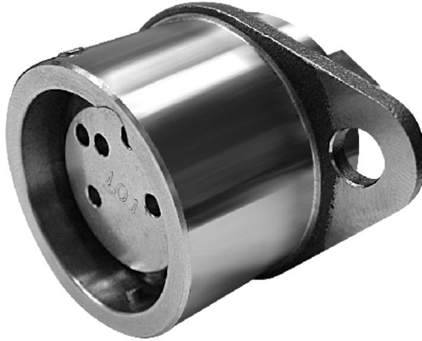
The MD Series Type SA1 and SA2 switchgear adapter interlocks have a 3/8" (9.5mm) square, 7/8" (22mm) long shaft that is controlled by the robust MD Series key. The mounting flange will accept two 1/4" (7mm) mounting bolts. Type SA1 and SA2 interlocks can be ordered with the shaft rotating clockwise or counterclockwise. Multiple degrees of rotation are available also.
